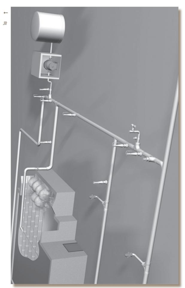
Valves isolate a section of a system, minimize areas out of service, and maintain protection in other areas. **All valves should remain open at all times!**
